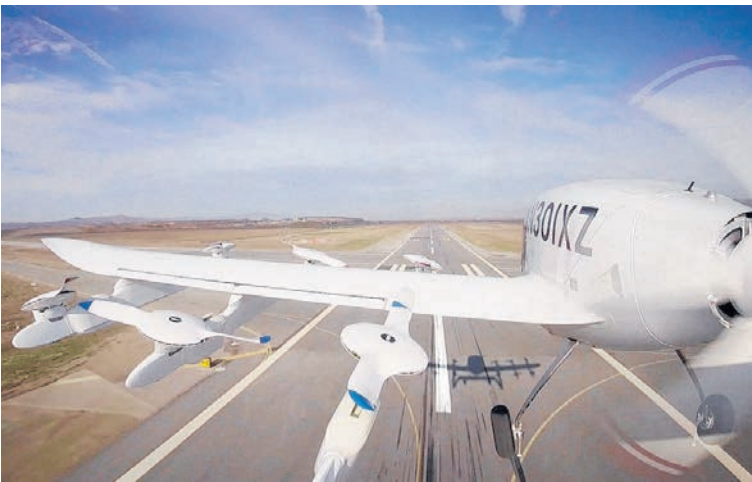
The self-piloted fan-powered Cora.
